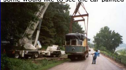
No. 10 is being gently lowered onto the trailer for it's five-hour move to Excelsior on 6-11-99.
