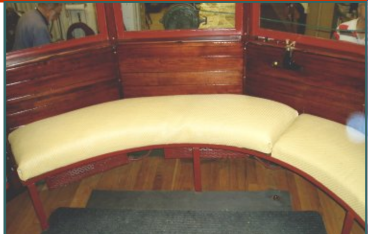
Here's the new rear seat on No. 265. In the upper right of the photo you can just see the new brass "clip" that will now be used to retain the rear brake handle in the stowed (non-operating) position while No. 265 is being operated from the front.
